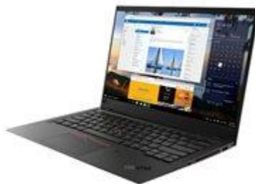
Lenovo ThinkPad X1 Carbon (6th Gen) - 14" - Core i5 8250U - 8 GB RAM - 256 GB SSD - US
